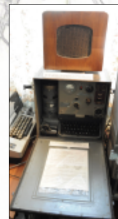
Hellschreiber machine from WWII. Tones were used to draw characters upon a moving drum.
